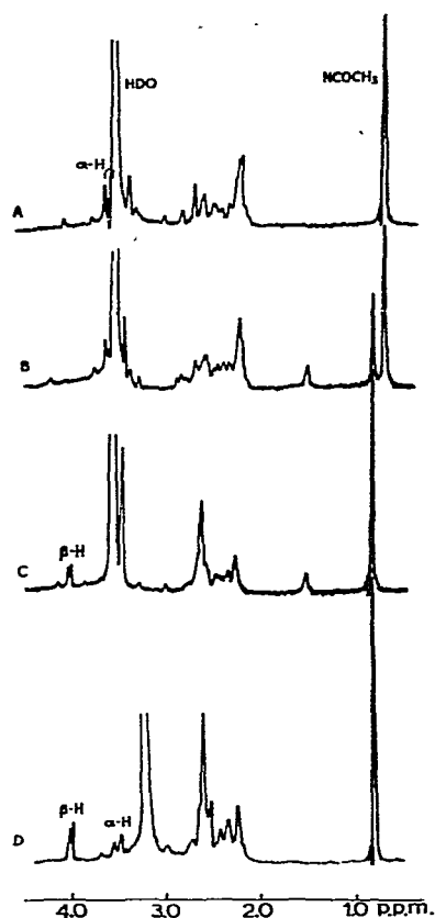
Fig. 1. N.m.r. spectra of (A) benzyl 2-acetamido-2-deoxy- \beta -D-glucopyranoside, (B) the enzymic digest 10 min after the enzyme addition, (C) 2 h after the enzyme addition, and (D) 2-acetamido-2-deoxy- \alpha,\beta -D-glucose.
